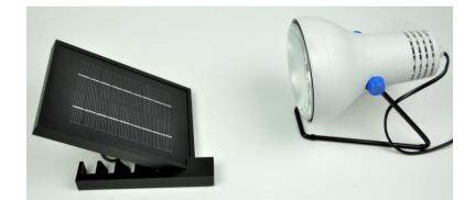
The angle of incidence can be varied by means of the stand. The following angles can be adjusted (printed on the stand):
