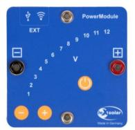
The PowerModule is a compact and intuitively usable voltage source. First, the attached power adapter has to be connected to a power outlet and to the top right input jack. The voltage can be chosen with the "+"- and "-" -buttons and will be displayed by LEDs. When the desired voltage is chosen, the voltage will be applied by using the yellow on/off- button. In case of a short circuit or currents greater than 2 A the PowerModule will switch off immediately.
