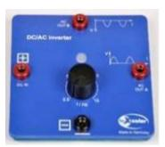
DC/AC inverters are used to convert the DC voltage of the solar module into an AC voltage to either feed the electricity into the grid or to operate customary domestic appliances in a smart-grid system. The leXsolar DC/AC inverter module does not produce mains voltage but an AC voltage with an amplitude of 2.5V and a variable frequency that can be adjusted with the potentiometer between 0.5
