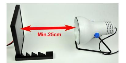
The solar module is adjusted against the lamp and stabilized with the stand. The minimum distance between the lamp and the solar module should be **25cm**.
