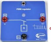
So called pulse width modulators do not load the accumulators continuously but with pulses of fixed frequency and different length. The ratio of pulse duration and pulse period – the so called duty cycle – determines how fast the accumulator is loaded. With this process one can ensure that the accumulator is kept on its maximum capacity as long as no consumer is connected. The advantage over the
