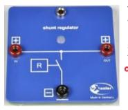
The shunt-regulator is a charge controller that short circuits the input voltage when reaching the charge end voltage to protect the accumulator from overload. It is a two-level controller with an upper switching threshold of 4.2V and a lower switching threshold of 3.6V. The working principle of the control LED is identical to the series regulator. Before starting the experiment, the capacitor should be loaded up to 2V to ensure the correct operation of the control LED.
